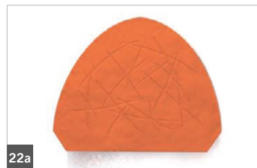
Fig. 22a: Preparing the base of the model (a) roughened for rigid mounting.
